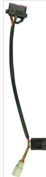
If you have a standard OBD reader you will need only the harness supplement to connect it with the ECU of the bike. If you don't have an OBD reader Rieju suggest use the KIT OBD READER WITH HARNESS SUPPLEMENT, this kit has been tested on Rieju bikes and its operation is guaranteed
