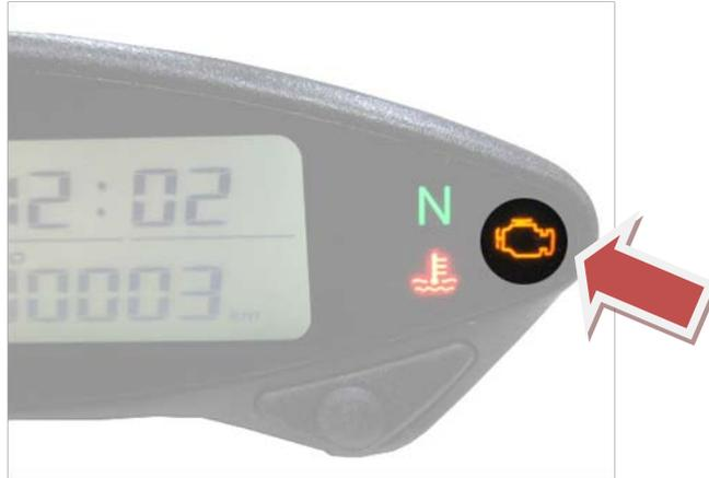
To know the cause of the failure you will need to connect to the ECU with a OBDII reader, this tool can be show the diagnostic Error and erase it, once the error has been erased the symbol on the dashboard will switch off, if after erasing the failure the symbol continues it means that the problem is not solved.
